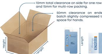
50mm clearance on ends when batch slightly compressed to allow space for hands.
